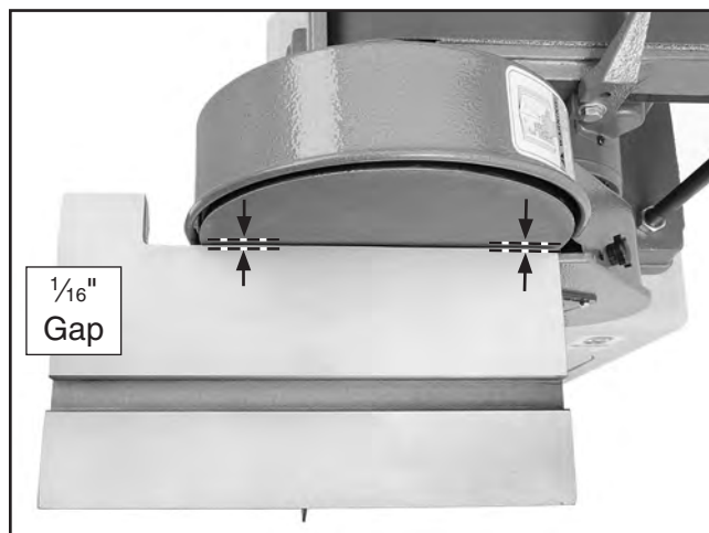
Figure 35. Correct distance between disc and work table.
